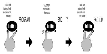
The display will then sequence as shown in the chart below. Tap the STEP button to advance to the next item in the list. Tap the LF button to select alternate values of that item. *Hold* the LF button to increase a numerical value; *tap* the LF button to decrease a numerical value. The shaded areas in the chart below pertain only to the Fuel Flow Option.
