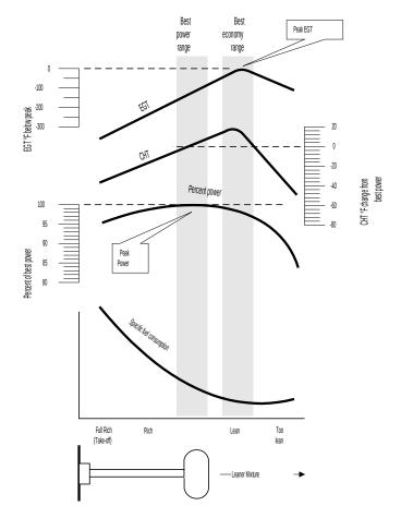
As the mixture is leaned, *EGT* rises to a peak temperature, and then drops as the mixture is further leaned. Peak *power* occurs at a mixture using more fuel than at peak EGT. Best *economy* occurs at peak EGT. Accurate leaning yields optimal engine temperatures. By being able to precisely adjust the mixture, your engines can produce either the highest fuel economy or maximum power, whichever you choose.
