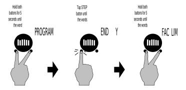
The display will then sequence as shown in the chart below. Tap the STEP button to advance to the next item in the list. Tap the LF button to select alternate values of that item. *Hold* the LF button to increase a numerical value; *tap* the LF button to decrease a numerical value. The shaded areas in the chart below pertain to the Fuel Flow Option only.
