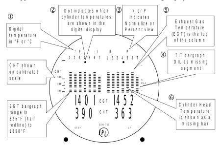
The following is a description of the analog display, from top to bottom. Numbers in circles refer to features in the above diagram.
