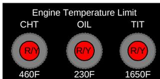
The lamp will light when the indicated temperature exceeds alarm limit. The limits for these alarms and warnings are preset by the factory for your type of aircraft and can only be changed at the factory. The yellow warnings are set as follows: CHT 45°F below redline, OIL 25°F below redline, and TIT 100°F below redline.
